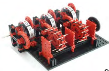
Reconstruction of a computing machine designed by Leibnitz in the 17 th century
