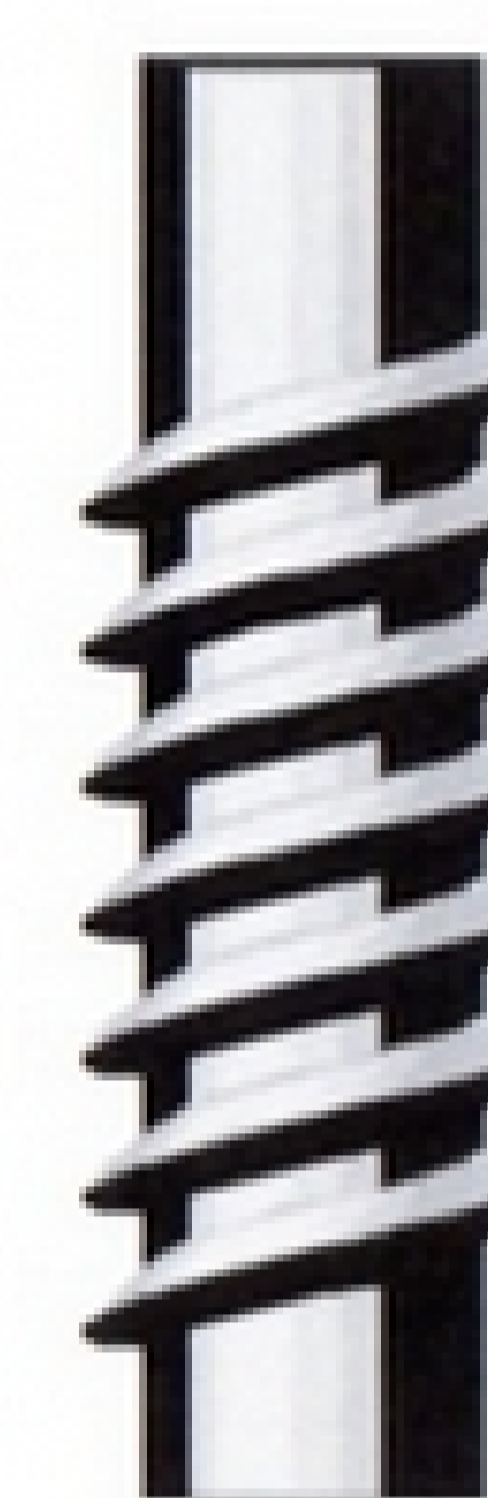
The ramp wrapped around the bar forms the screw.
